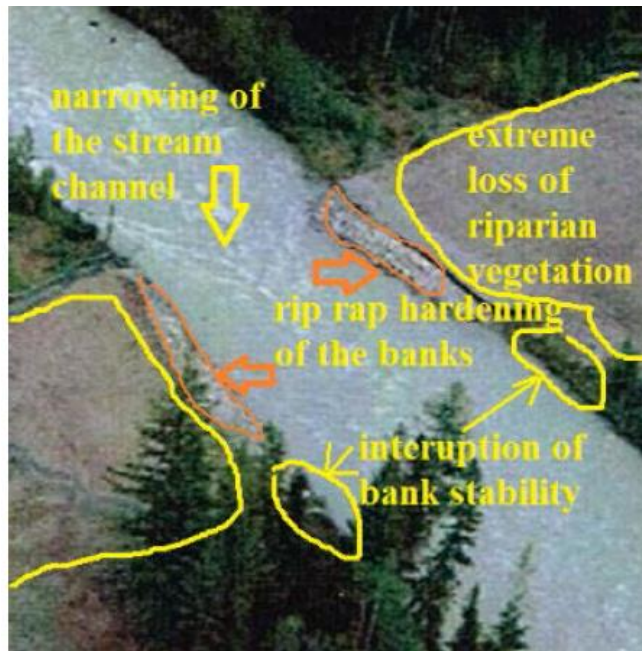
Extensive damage to the stream bank and riparian areas at the Moose River Trans Mountain pipeline crossing as a result of the Anchor Loop TMP project, c.a. up to 2008. For all intents-and-purposes, and from a fish-habitat perspective, this stream crossing can be viewed as a "biological scorched-earth zone". Figure adapted (notations on photo, SRES additions) from May 19/20, 2015 TMP information meetings (presentation powerpoint by Calum Bonnigton, GeoMarine Consulting).
