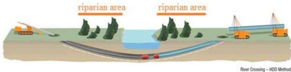
Figure 1 Generic example of a trenchless method of stream crossing. Note that the riparian areas, in this diagram, are largely protected as a result of this method.
